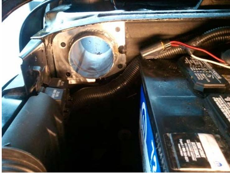
Take the supplied 90° Rubber elbow and one stainless steel hose clamp and insert them down through the opening in the cowl. Secure them to the backside of the firewall intake bracket. Be sure to position the elbow so that it lines up with the hole that has been cut in the top of the cowl.
