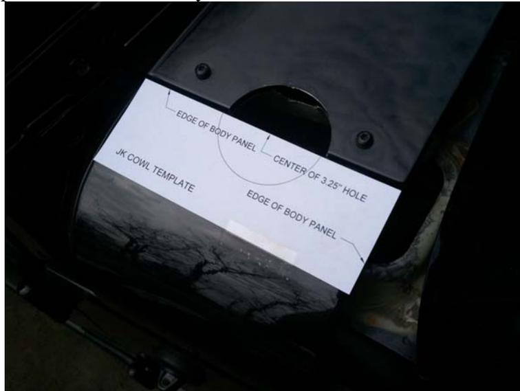
With the template in place, mark the center of the 3-1/4” hole that you are about to cut with a center punch. Now, using a 3-1/4” hole saw, carefully cut the hole in the cowl. You will be cutting through several layers of metal. Take your time to insure a clean and accurate cut.
