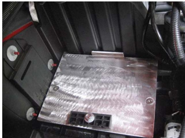
Now turn your attention to a small unit positioned next to the battery tray that has several black airlines attached to it. We are going to lower this unit approximately one inch. Pull up on this unit and slide it off of its mounting post. With a utility knife, shave both sides of the mounting post to allow the unit to slide down further. You will also need to remove approximately one inch off the top of the mounting post. Now reinstall the unit at its new, lower location.
