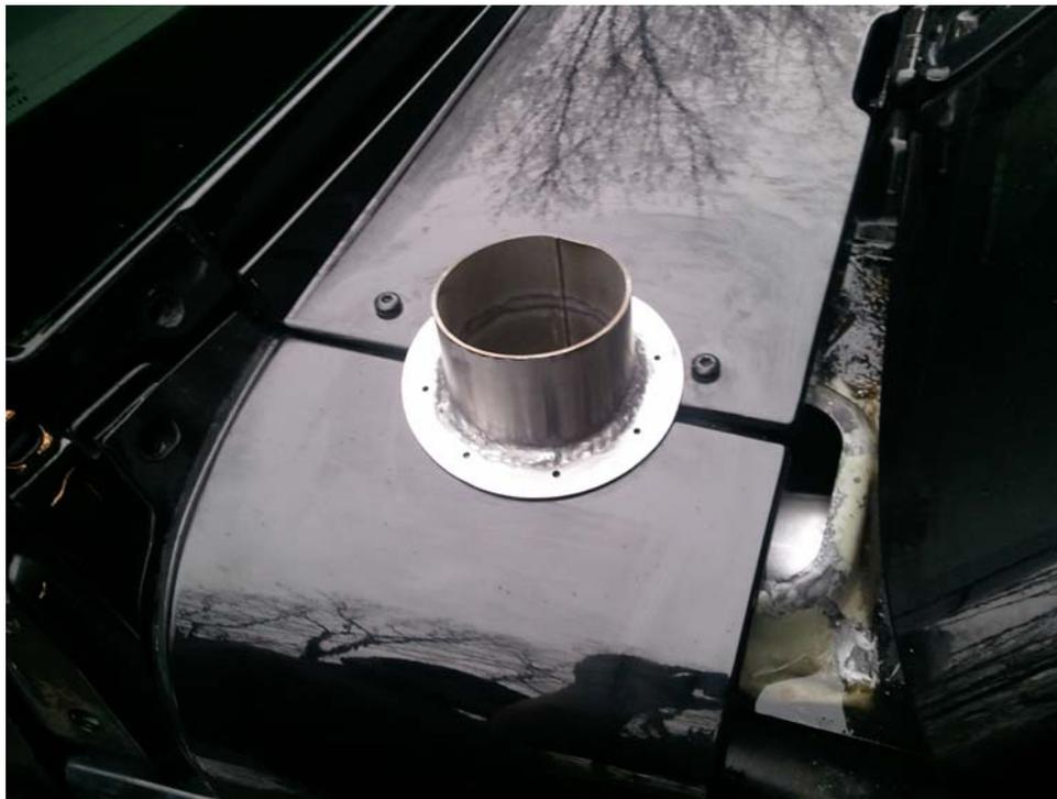
Now take the supplied rubber gasket and fit it onto the lower portion of the cowl snorkel unit and insert the cowl snorkel unit through the cowl into the rubber 90. Position it so that it fits the contour of the cowl. Once in position proceed to drill the eight 1/8" holes into the cowl and attach with the supplied stainless steel rivets. Take your time and do a nice job.
