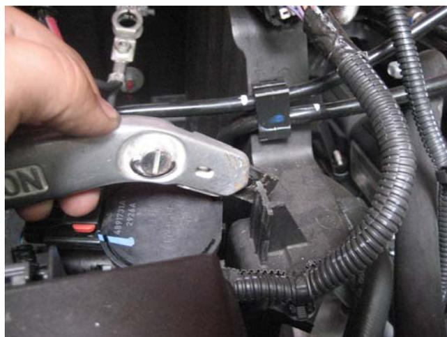
Remove the factory wiring harness from its post in the upper left-hand corner of the firewall. This will allow you to clearly see the area where the new intake will be routed through the firewall.
