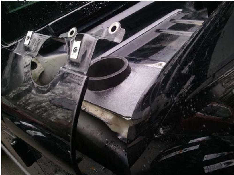
Now it's time to install the firewall intake bracket. Run a bead of 100% black silicone on the backside of the firewall intake bracket and position it on the firewall. Proceed to rivet the firewall intake bracket in place with four stainless steel rivets.
